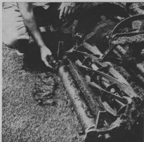
Wet clippings that accumulate on roller change height of cut, emphasize desirability of mowing when grass is dry.
