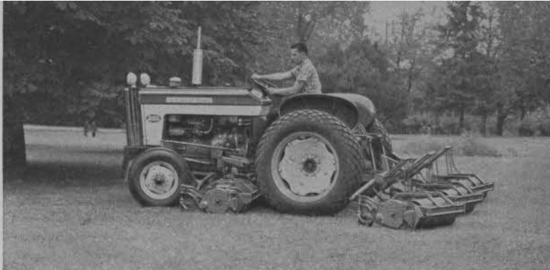
45 hp* International 340 Utility tractor with 5-gang mounted reel mower.
