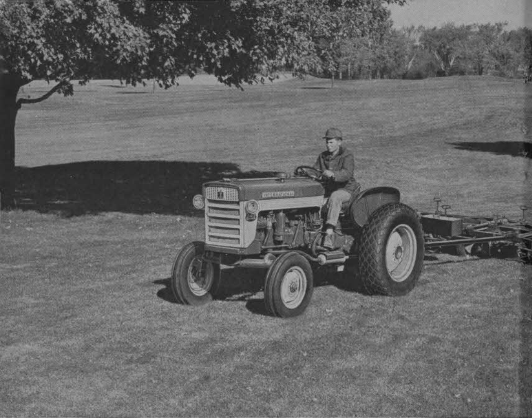
38.5 hp* International 240 Utility tractor with 7-gang reel mower.
