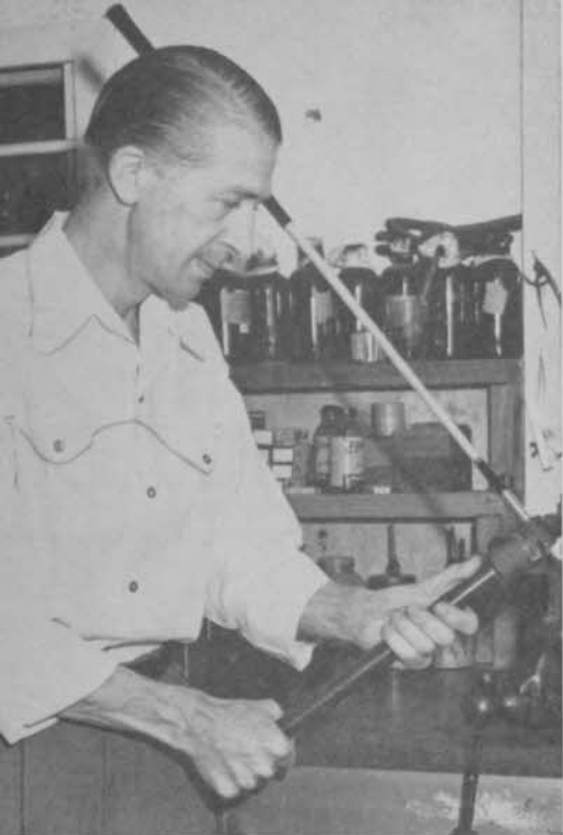
The author, who teaches club repair courses at the PGA Business School, is shown changing the lie on an iron club.
