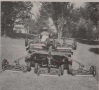
AS A 5-UNIT MOWER , machine has overall width of approximately 12 ft. 2 inches, cutting width of about 11 feet.
