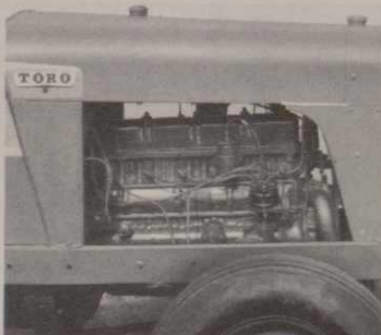
POWERFUL 6-cylinder industrial engine is rated at 130 hp—plenty of reserve power for climbing grades.
