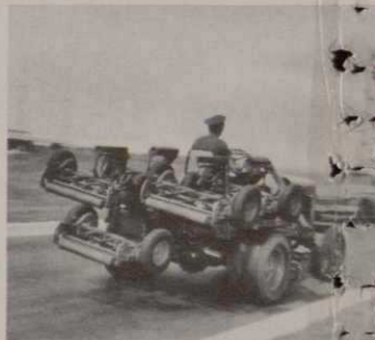
GANGS NEST AND LOCK in transport position so Parkmaster may be safely operated at speeds up to 30 mph.
