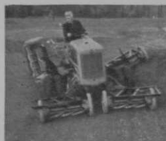
Worthington Model F with "Wing-Lift" hydraulic control offers either three, four or five units.
