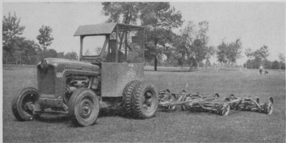
Drivers on all tractors at the Montreal, Que., municipal course are protected by a homemade wire cab. This is a very heavily played course.
