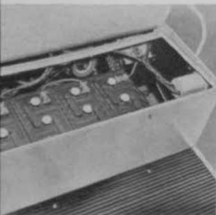
These 200-ampere-hour batteries give more travel between charges. Properly engineered circuits reduce electric resistance to a minimum—put all the current to work driving the car. There's less stalling of cars on the course with the Worthington "Champ."
