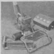
**DIS-ASSEMBLED MOWER** shows simplicity of design. Supporting fork, attached to traction unit, takes weight of grass catcher. Cutting unit mounts independently.
