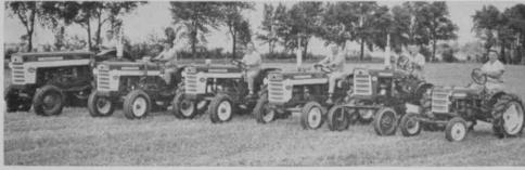
These six International Harvester tractors are part of a complete new line of 12 commercial and farm tractors in six power sizes. From (I to r) they are: International 560, 72 est. ehp; the 460, 61 est. ehp; the 340, 45 est. ehp; the 240, est. 38 ehp; 140, 28 est. ehp; and the International Cub Lo-Boy, 12.8 est. ehp.
