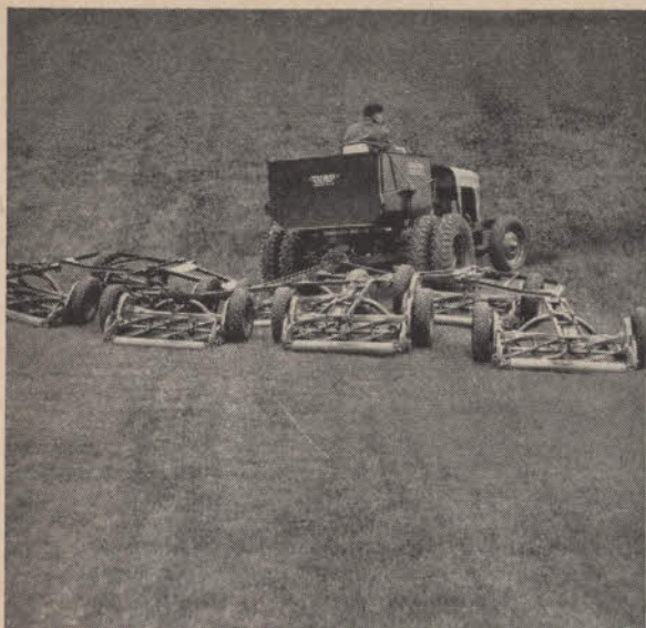
FAIRWAYS? 7-unit Universal Frame (shown with Toro General Tractor) mows a swath approximately 17 ft. wide.
