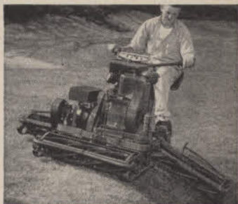
UNEVEN GROUND? Hinged "wing" reels of the 76-inch Toro Professional hug ground contours.
