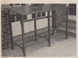
Registry & Scorecard Marking Table is 6' wide and 2'-6" in depth — 3'-1" high in front and 3'-5" high in back. Table is designed to serve two or more users at one time, and is constructed of twelve gauge steel framing with a tempered hard board to top give a smooth, even writing surface.
