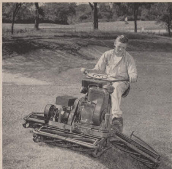
UNEVEN GROUND? Hinged "wing" reels of the 76-inch Toro Professional hug ground contours.
