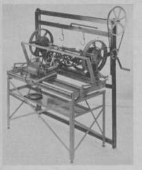
Fastest most accurate lawn mower sharpener ever used. Sharpens all mowers, hand, power, greens mowers or fairway units. Bed knives may be sharpened without removing from mower. Full floating rails may be turned as desired, retain perfect alignment. Grinding head feeds in or out and will hollow or flat grind.
