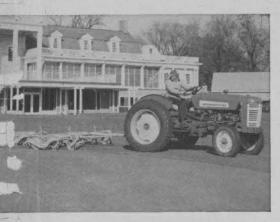
International 330 Utility, for dependable mowing power on a small equipment budget. Easily handles 7-gangs; 60-inch rotary or Hammer knife; or 7-foot cutter bar mowers with minimum fuel. 40 engine hp.\*
