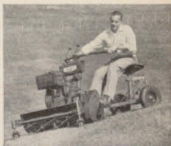
TEES? Standard six-blade reel on the 30" Park Special has high frequency of clip. Sulky optional.
