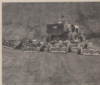
FAIRWAYS? 7-unit Universal Frame (with Toro General Tractor) mows a swath approximately 17 ft. wide.
