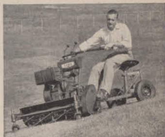
TEES? Standard six-blade reel on the 30" Park Special has high frequency of clip. Sulky optional.
