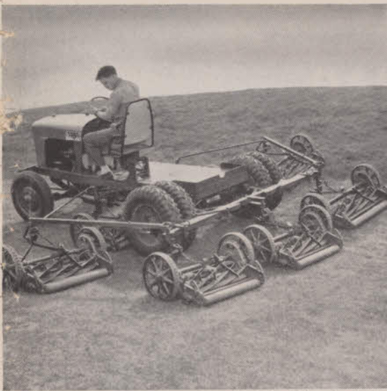
FAIRWAYS? Two gangs placed ahead of the drive wheels give a shorter turning radius with the 7-Unit Master Frame.
