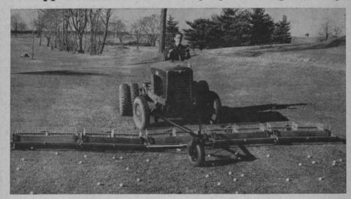
This amazing new machine has rollers of durable pliable rubber which pick up the balls very lightly . . Has no wheels nor circular flanges to wear or mar the balls . . Easy on turf, no blind spots . . The entire  $44^{\prime\prime}$  of one unit is the picking surface.
