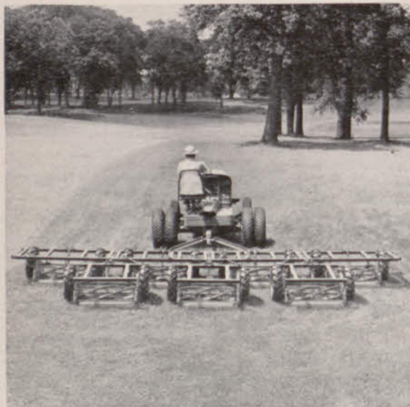
FAIRWAYS? Seven-unit Toro Roughmaster Frame (shown with Toro Bullet Tractor) mows a swath 16 ft. 6 in. wide.
