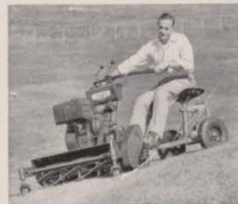
APPROACHES? Traction-wheel differential of 30-inch Toro Park Special gives high maneuverability.
