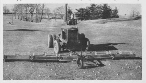
This amazing new machine has rollers of durable pliable rubber which pick up the balls very lightly . . Has no wheels nor circular flanges to wear or mar the balls . . Easy on turf, no blind spots . . The entire 44" of one unit is the picking surface.
