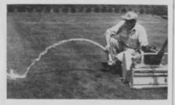
Point Products Corp., West Point, Pa., the new machine is self-propelled and features a 24-in. long cellulose sponge roller which absorbs moisture as it rolls across the grass. The specially fabricated Du Pont sponge, which helds up to 20 times its weight in water, is squeezed dry by a wringer and the water whisked to a removable sump pan.
