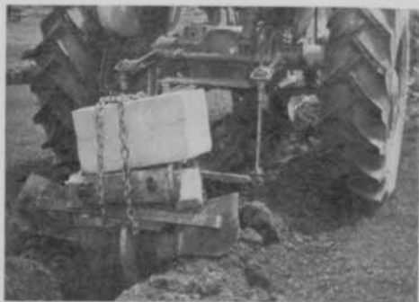
Trench was dug with homemade trencher built on sub-soiler and drawn by a tractor.
