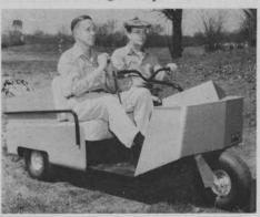
an automobile universal joint, reinforced disc brakes and a safety switch for forward and reverse operation. Another change includes a microswitch that controls speeds more fully.
