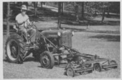
ing, grading or snow removal. It has many uses in course and park maintenance, being rated in a power class between walking type and larger utility tractors. Loader, air compressor, earth auger, three cu. ft. concrete mixer and insecticide sprayer or duster are among the implements that can be used with the Lo-Boy.
