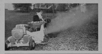
Is just the thing for golf course leaf disposal, Vacuums up, cuts into fine mulch, returns leaves to ground in single operation. Tractor-drawn, 6' 5" pickup cleans up to 30 acres in 8 hr. day. 25 HP power unit shown, smaller models also.
