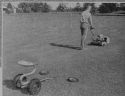
Transport wheels and sulky can be attached or detached in seconds, without tools.
