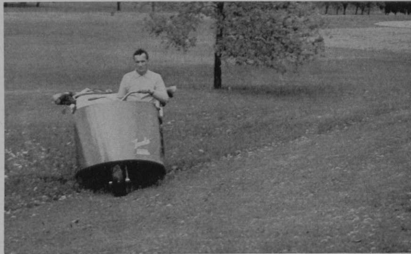
Go up hill zig-zag, reducing the grade and avoiding danger to turf.
