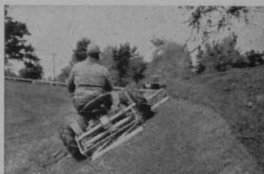
LOW CENTER OF GRAVITY—HERE IS AN 83% (40°) SLOPE — HERETOFORE CONSIDERED IMPOSSIBLE.
