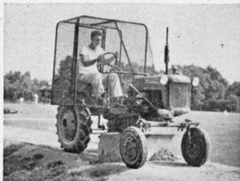
GRADES GROUND WITH DOZER BLADE
