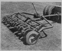
with saw-toothed knives, adjustable in penetrating depth from 2-3-4 inches. These saw-tooth knives are shaped so as to perform a definite slicing action in controlling long step grasses and cutting endless number of slits 2 in. long in turf without tearing the surface.
