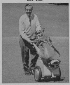
Henry Cotton has been testing this electric bag cart for a year on British courses. after the device had four previous years of development. It weighs 85 lbs., does two rounds on a battery charge, has regulator for speed and pulls a player up hills.
