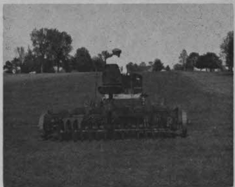
Jim Morrison's vertical mower for cutting crab grass seed heads. Morrison used old rotary hoe and cutters from plows.
