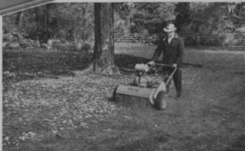
Jacobsen Leaf Mill 30-inch width — 6 hp. engine
