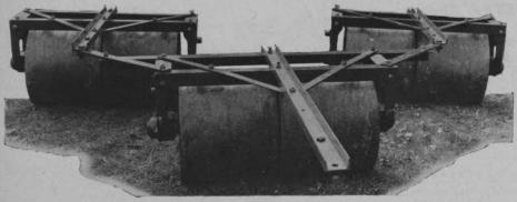
SPECIFICATIONS — Individual sections are of fine cast-iron, beveled on the outer edge, 21 in. diam. x 18 in. width. End frames are of heavy cast-iron, with dust-proof bearing housings, furnished with Zerk fittings. Sections run on cold-rolled steel axles, supported in Maple bearings, which are replaceable.
