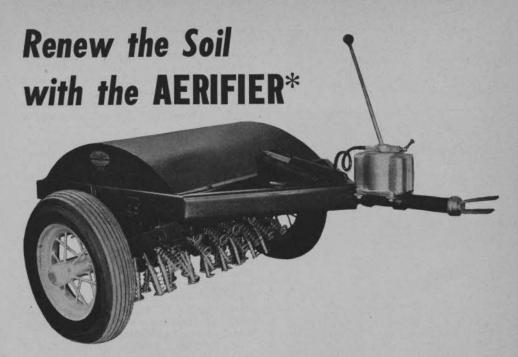
Only the Aerifier produces real root zone cultivation. The Aerifier scoops out soil cores. Movement of the curved spoons stirs the soil in the root zone. This important "cultivating action" allows new roots to grow into the loosened soil around the openings.
