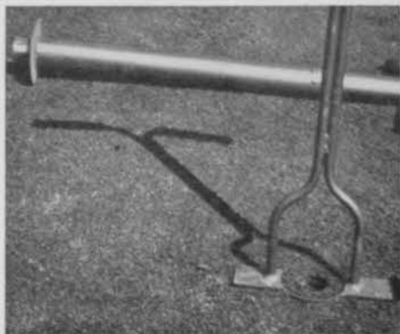
2. — 4-in. West Point plugger in place to remove plug for planting.
