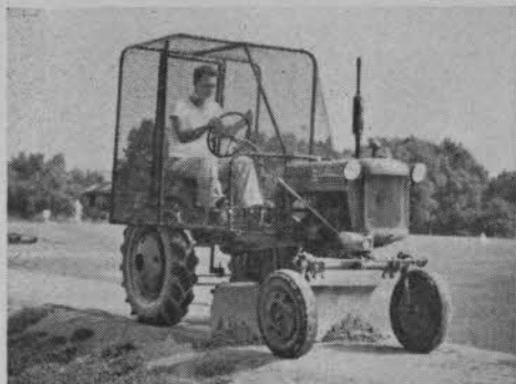
GRADES GROUND WITH DOZER BLADE
