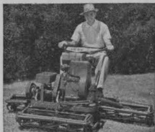
**TORO "PROFESSIONAL."** Cuts 15 to 20 acres per day with 76" swath. Convertible to 30" swath. "Out-in-front" reel cuts close. Forward and reverse transmission. Wisconsin 7½ h.p. engine.
