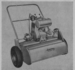
transmission. Separate mill and traction clutches — disc type with controls on mill handle. The machine is designed so that sticks, stones, etc., are ejected without any damage to the machine. Operator can keep rolling right over grounds where twigs are mixed with the leaves. For descriptive literature on this new unit, write Jacobsen Manufacturing Company, Racine, Wis.
