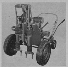
stronger one-piece cast ram housing, more positive chain and belt alignment, and uniball joints on the walking beam are included in the improvements. Change-over kits are available for all previous models. Full particulars from the manufacturer.
