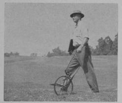
Measuring distances now as easy as walking. Using a Rolatape Model 400 measuring wheel, Bill Stewart, supt., Hillcrest CC, Los Angeles, checks score card distances on the course. The wheel may be used to measure any distance on any surface - a counter in plain view of the operator at all times records distances up to 100,000 ft. directly. It has special significance in determining areas of greens that have to be fertilized or treated chemically.
