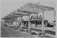
here illustrated. The steel standards are gracefully curving, the joists and girders are made of dressed lumber and the top of transparent, corrugated fibreglass in various colors. The players stand well in front of the ample room between the standards. The canopy was designed and installed by Chain-Link Fence Corp., Chicago, manufacturers of the Chalinko Golf
