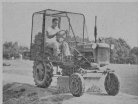
GRADES GROUND WITH DOZER BLADE
