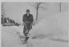
has a 17 in. plowing swath, is powered with a 2½ Briggs and Stratton 4-cycle engine, is easily pushed and throws snow 10 to 15 ft. to the right or left of the machine. Snow is collected through a screw-action rotor which propels it up and out of the directional shute thus making it impossible for snow to be compacted in front of plow and reducing tendency of the mechanism to freeze in very cold weather.
