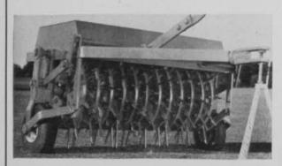
The spiking assembly is quickly detached from the frame by removing four bolts. Spoons easy to replace. The tractor drawn Perry's Greens Spiker is transported on its heavy duty rubber tires with lift bar handy for operation from driver's seat.
