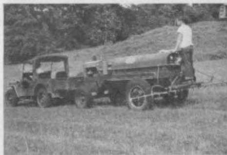
Spraying rough in late June with 2, 4-D at Moraine. Supt. Orville Young uses 1 lb. of 2, 4-D to 75 gals. of water per acre at 15 lbs. pressure.
