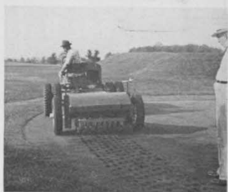
Aerifier on green, showing raised turf around each hole. Rolling lightly in opposite direction following removal of plugs puts green in shape for immediate play.
