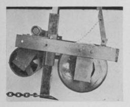
This is the mole-drain assembly which fits into the Aerifier frame. The sharp disc at the front cuts a slit so the arm on which the bullet and chain are mounted will not tear the turf. The roller in the back presses down turf at edges of slit. The extent to which it marks the surface is shown in the picture below.
