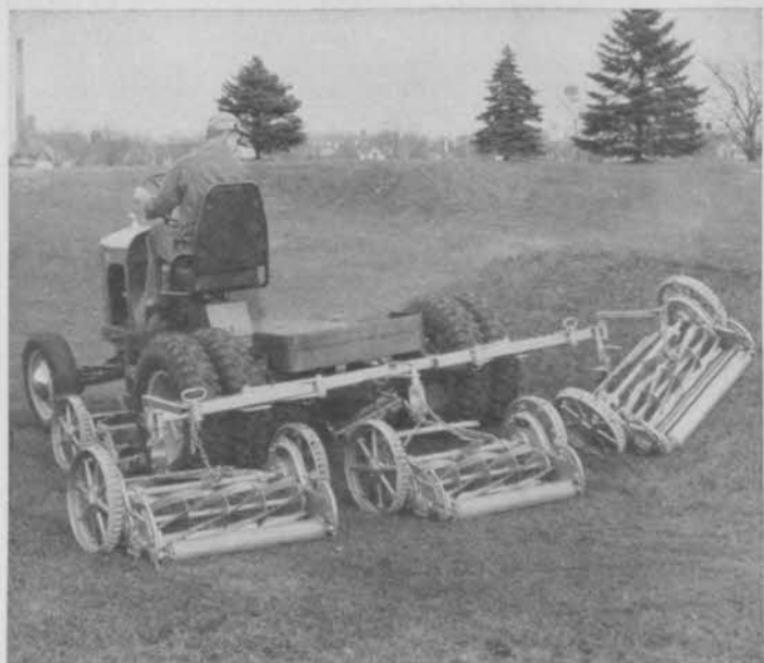
TORO MASTER TRACTOR with underslung gangs which mow ahead of rear wheels for smooth, ridgeless cut. One of Toro's great line of turf maintenance tractors available in various sizes and models with dependable Toro Spartan Gang Mowers in underslung or trailing type frames.
