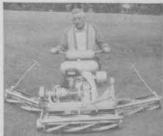
TORO PROFESSIONAL. Cuts up to 25 acres per day with 76" swath. Convertible to 30" swath. "Out in-front" reel for close cutting. Forward and reverse transmission. Toro 4½ h.p. engine.
