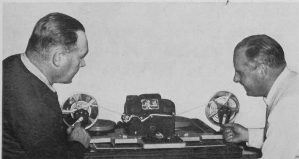
Bill Gordon, left, and Jules Platter, right, check on film of golf swing as shown on screen of Video Instructor. Any frame of film can be stopped and studied. Film can be run forward or in reverse at any speed.
