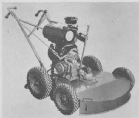
The Toro Whirlwind Grass King rotary blade type mower has a 31-inch cutting width, a Briggs & Stratton 4 cycle motor and a cutting capacity of 6 acres per day.
