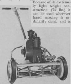
especially adaptable to cutting bunkers or steep terraces. The Sportlawn also has many of the features found on higher priced machines including finger-tip clutch and throttle controls, adjustable cutting height, semi-pneumatic tires, sectional rol-
