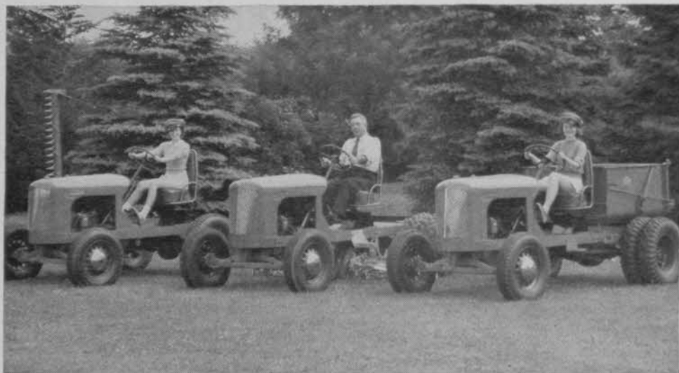
Three popular Toro turf-maintenance tractors designed for dependable low cost operation. Left, Toro Bullet with Sickle bar, a lightweight favorite, exceptionally maneuverable and easy to operate. Center, Toro Master tractor with gangs underslung to cut ahead of rear drive wheels. Right, Toro General all-purpose tractor with dump box.
