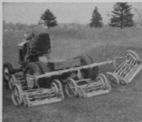
Toro Master Tractor with underslung hitch. Gives you a finer, smoother mowing job with no ridges or uncut strips because two mowers cut in front of the rear drive wheels. The Master Frame handles 3, 5, or 7 gangs of mowers and cuts a fine, even swath up to 17'2" wide.
