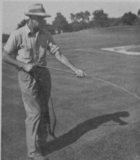
Ray Rolf demonstrates his sub-irrigator. Small stream of water flowing through welding tip brazed on end of tube accounts for ease of inserting tube in most compact soil generally found beneath localized dry spots.
