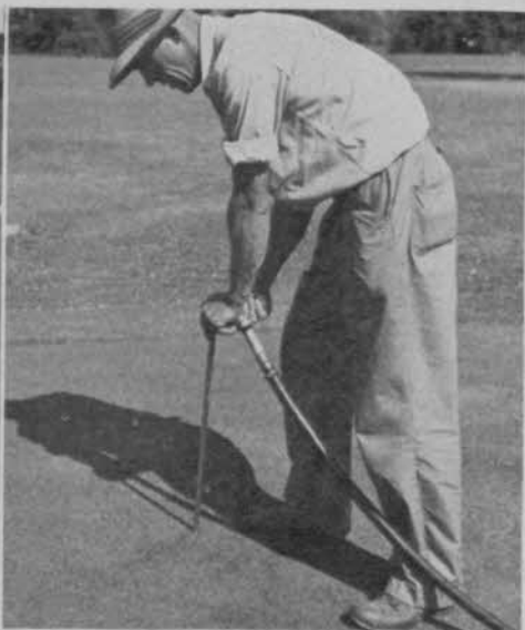
Ray Rolf demonstrates his sub-irrigator. Small stream of water flowing through welding tip brazed on end of tube accounts for ease of inserting tube in most compact soil generally found beneath localized dry spots.
